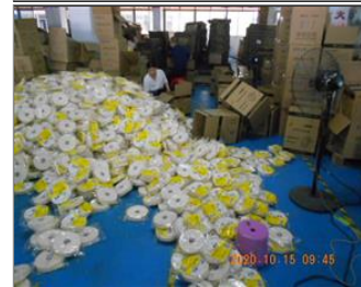
Photo of non-conformity NC Evacuation route was blocked 1.JPG
